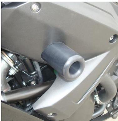
Hotbodies Racing frame sliders serve the purpose of mitigating damage to the motorcycle. Although statistics have shown that frame sliders reduce damages to the frame, cases, swing arm, and levers there is no guarantee that this product will eliminate damage all together in the event of a crash.
