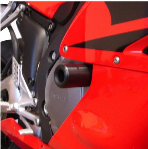
Hotbodies Racing frame sliders serve the purpose of mitigating damage to the motorcycle. Although statistics have shown that frame sliders reduce damages to the frame, cases, swing arm, and levers there is no guarantee that this product will eliminate damage all together in the event of a crash.
