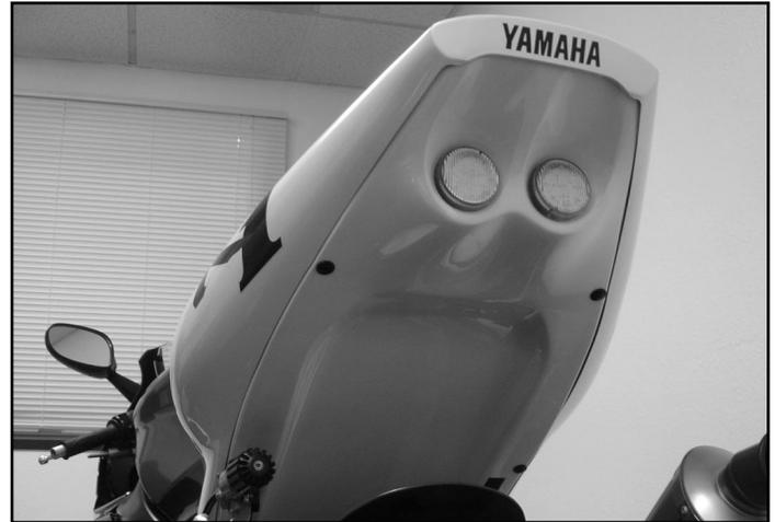
7) Re-install stock tail section leaving the mounting hardware loose to allow the undertail to shift into position. Insert undertail left side first, then right side, be careful not to crack or scratch undertail. Use your stock plastic screw rivets to hold undertail in place, start from the top and work your way to the bottom. Tighten all hardware on the tail section, attach seat. Your done!
