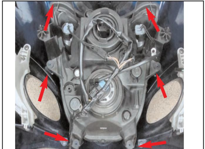
**2)** Remove 6 phillip head bolts, holding the headlight to upper fairing. Then remove headlight from your fairing.
