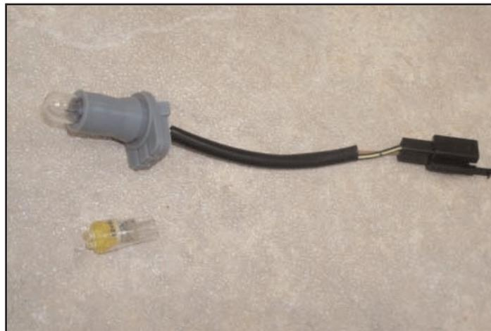
**5b)** To install signals in headlight, remove running light plugs from headlight housing. as pointed out in photo 5a. Replace stock bulb with provided amber LED marker, plug running light back in to headlight housing and re-wire.
