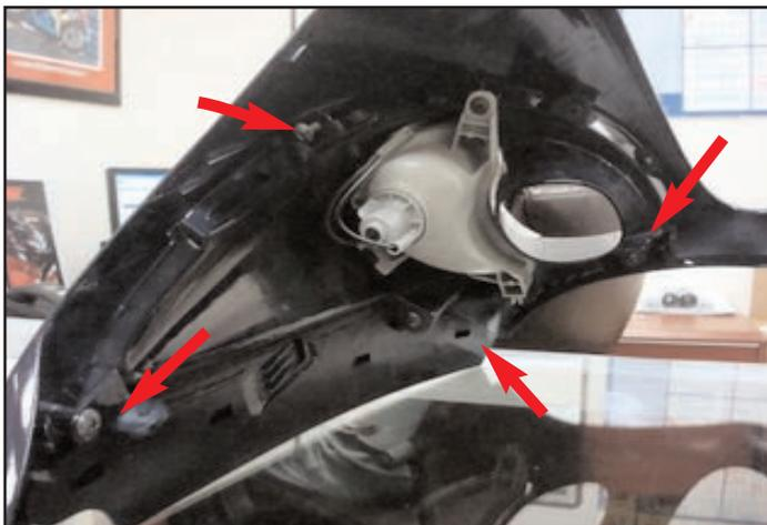
**3)** Once headlight is removed, you can now access and remove the 4 phillip head bolts, holding the stock cover and turn signal to the upper fairing.
