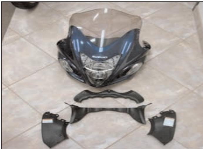
**1)** Remove entire front upper fairing. Including headlight, mirrors, windscreen, and dashboard pieces for easier installation of air scoops.
