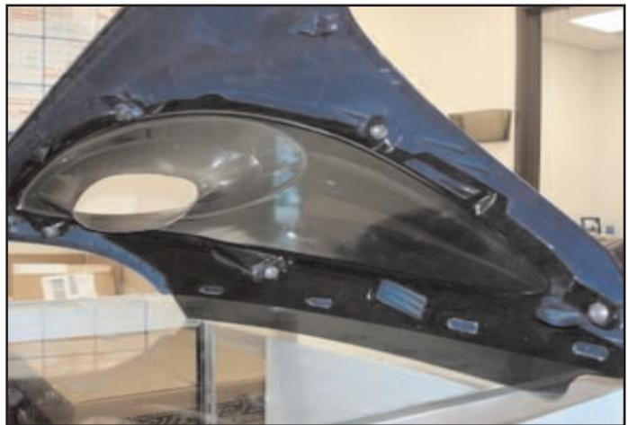
**4)** Once stock cover and turn signal is removed, install Hotbodies air scoops. Re-use phillip head bolts to secure scoops to upper fairing.
