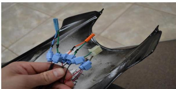
11) Prepare HBR undertail for installation. Connect your factory wiring harness to the undertail. Use wiring instructions down below. Note (you can also drill out your undertail for the license plate at this time, but be sure to check the position for clearance with the rear tire with suspension travel.)
