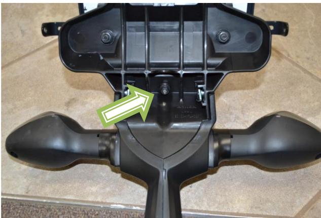
5) Also remove the 8mm nut behind the reflector and remove the cover hiding the turn signal wires within the mudflap.
