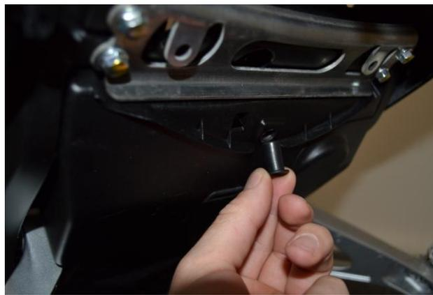
10) Insert rubber well nut from bottom up through the battery box, so the fat part is underneath the tail.
