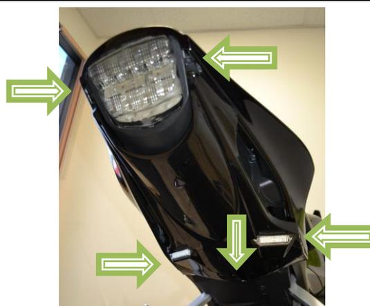
12-B) Pictures shows undertail in position for final installation, arrows mark mounting tabs and fastener.
