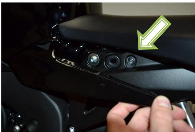
1) Remove side covers to access phillips bolts behind them to take off the rider seat. Also remove the passenger seat.
