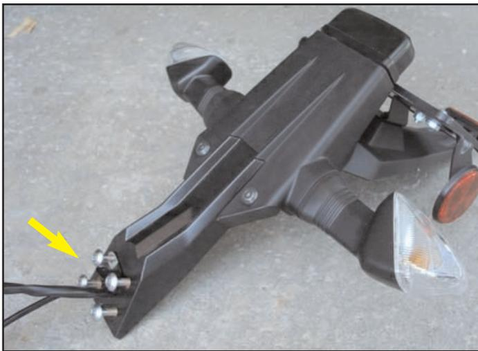
**1)** Remove seats and proceed to undo mounting bolts for tail section. Remove 5mm. hex bolts to undo mudflap (as pointed out), Disconnect signal light and license plate light wires to remove mudflap completely.
