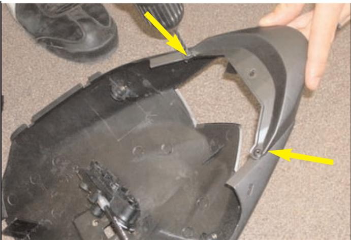
**3)** Drill out the two rivets that hold on the top end of the tail section to remove top piece (as shown in photo). Separated top end piece will bolt on to new undertail with nuts and bolts supplied.
