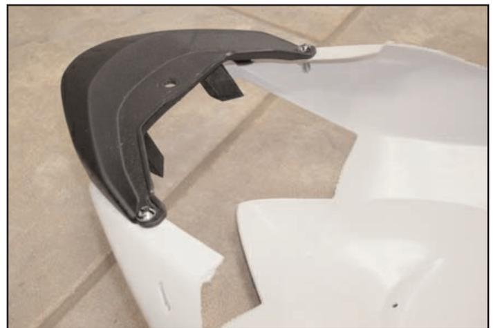
5) Trim inner tabs of tail section as seen in Fig. 2. Closer view in Fig. 3.
