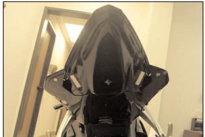
7) Re-install stock tail section with all stock bolts and hardware. \*Note tail light will not bolt up to the new undertail, when everything is securely mounted, taillight will be snugly fitted between new undertail and sub-frame. Re-install seats and your done!
