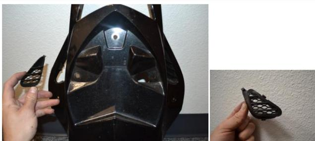
7) Remove the OEM vent inserts by pinching in the three release tabs then pulling out the vent. \*Be very careful not to break them\*
