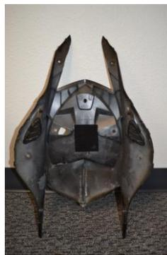
6) Separate the stock undertail from the tail section & the tail light. Be very careful not to break the tabs along the edges of undertail and tail section. Easiest way is to start with the round tabs in the front and then work your way backwards.
