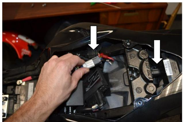
2) Unplug the electrical connector from main harness & also unplug the tail light.
