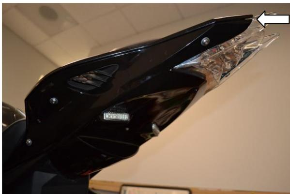
11b) \*Note there may be a 1-2mm gap at the very tip of the undertail where it meets up with the tail section. This can be adjusted during installation & is normal.
