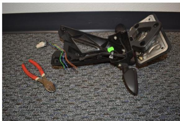
8) Wiring instructions: Cut off the OEM plug connector for your turn signals & plate light. Cut about half way down your OEM mudflap, this will give you plenty of room to run the wires nicely.
