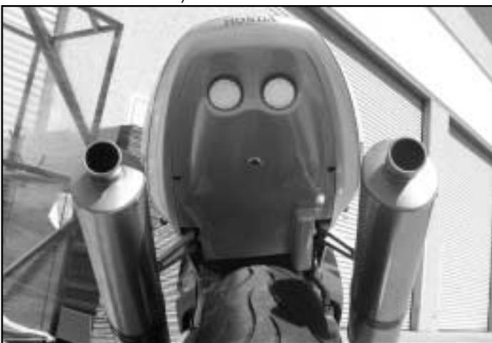
6) Inset lock into undertail using stock lock mounting clip, make sure the lock is in the correct position with the lock cable arm to function properly. Insert undertail left side first, then right side, be careful not to crack or scratch undertail. Use your stock plastic screw rivets to hold undertail in place. Attach lock cable to lock, check movement, adjust if necessary. Tighten all hardware on tail section, attach seat.
