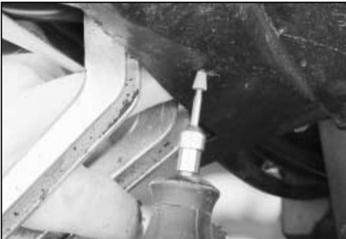
5) Replace all bodywork with fasteners loosely installed, mount undertail, notice at bottom of the tray there are 2 holes, mark and remove tray, then drill holes in battery box
