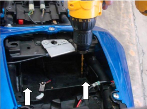
7. Drill out pop rivets through storage compartment, this will hold the pieces together, and will be the mounting location for your license plate.
