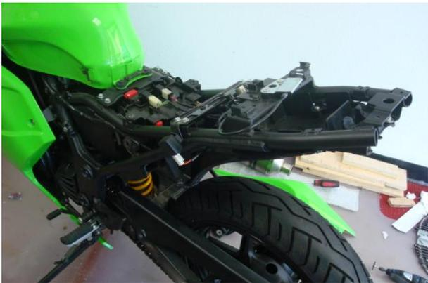
1. Remove seats and proceed to undo mounting bolts for the tail section. Also remove passenger foot pegs. Disconnect signal light and license plate light wires to remove tail light and mud flap completely
