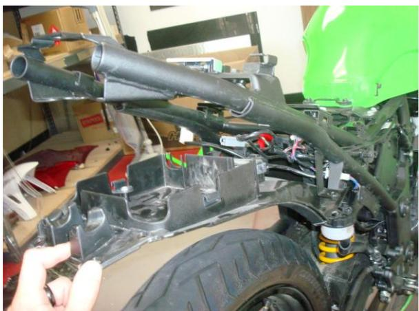
3. Remove bolts holding battery box to sub frame, to allow for easier access to trimming of battery box. Battery box will hang down.
