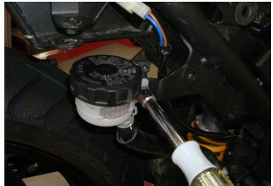
2. Remove bolt holding rear brake reservoir, and move reservoir out of way for installation. Make sure brake reservoir is upright to prevent any leaks. Also place cloth over reservoir bracket to prevent from scratching undertail during installation.
