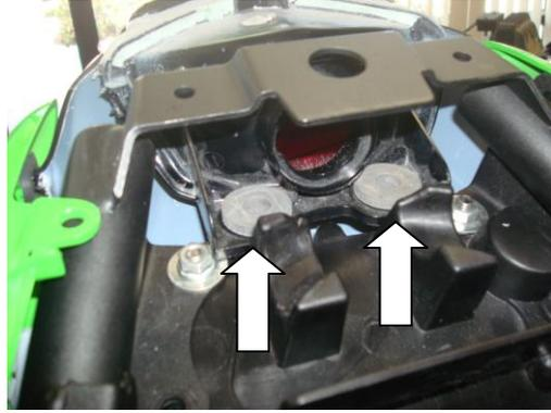
6. Once undertail is mounted on the sub frame, and battery box is bolted up; flip back part of tail light so that it rests on top of battery box. Once the undertail is secured the tail light will be pressed up against the battery box firmly and should not move.
