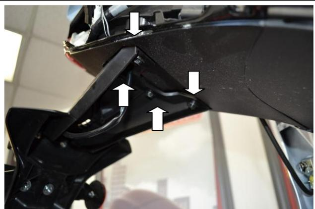
10. Remove the 4 bolts that hold the mud flap to the bike.
