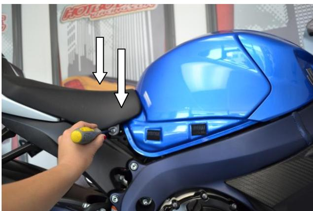
3. Remove the 2 bolts that are holding the front seat to the frame.
