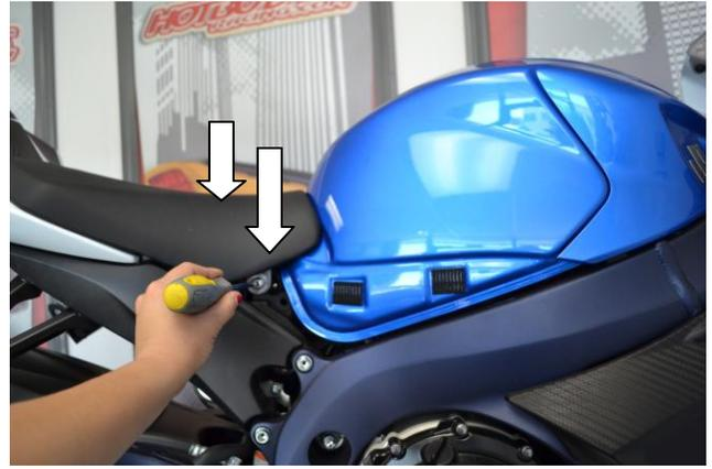
18. Reinstall the front seat, tightening the 2 bolts.
