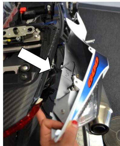
8. Pull right side tail fairing, and disconnect the electrical. Remove from bike completely.
