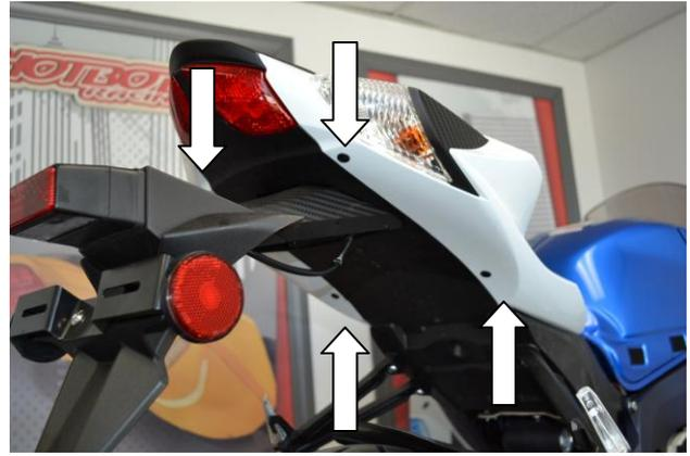
6. Remove the 4 pop rivets that are located on the underside of the side tail fairings.
