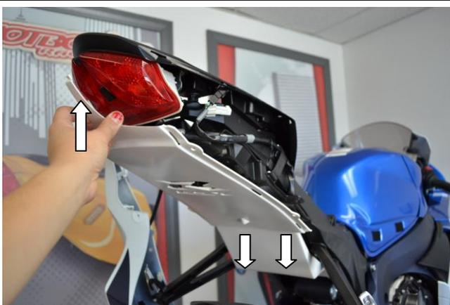
13. Install the new Hotbodies Racing undertail. The tabs at the bottom will be located between the battery box and bolts. The top will clip into place.
