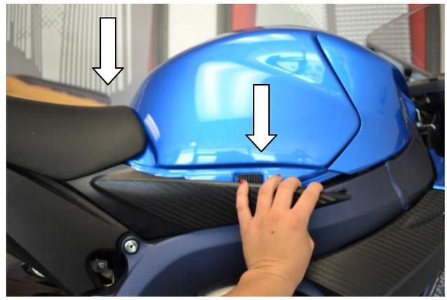
2. Remove the black fairing pieces from each side of the tank/ front seat, being careful not to break the tabs.
