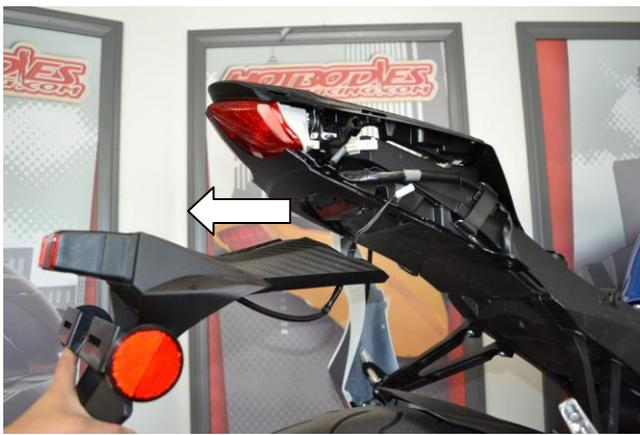
11. Pull the mud flap to remove completely from bike.
