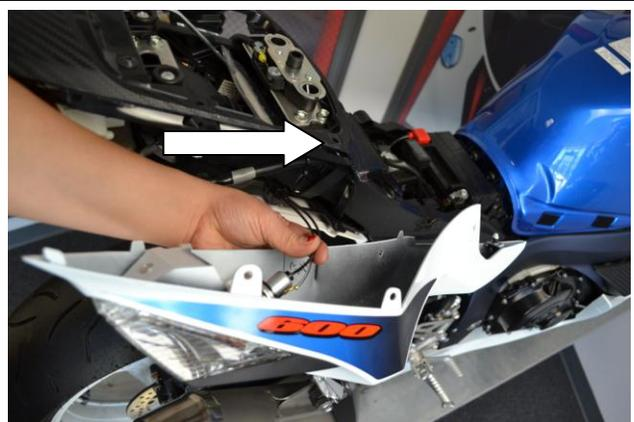
14. Reinstall the side tail fairings, and connect the electrical.
