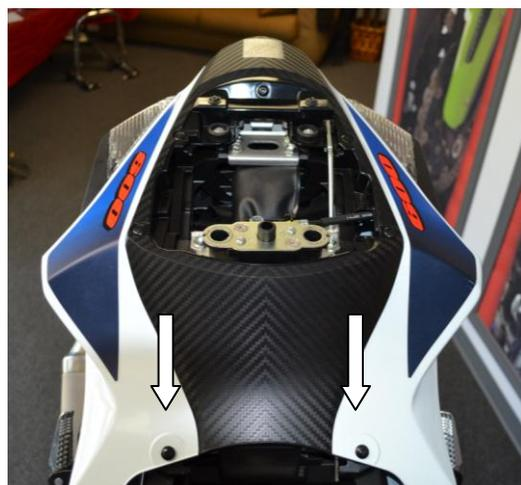
4. Remove the 2 screws that are holding the side tail fairings to the bike.
