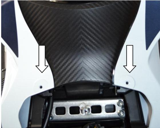
17. Reinstall from 2 screw located on the front of the side tail fairings.
