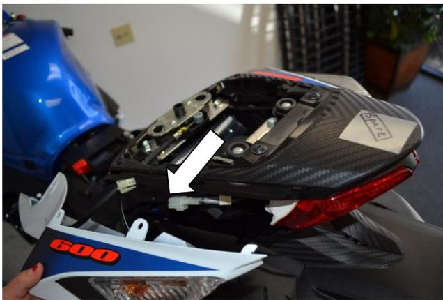
7. Pull the left side tail fairing piece, and disconnect the electrical. Leaving the lock mechanism attached let fairing hang.
