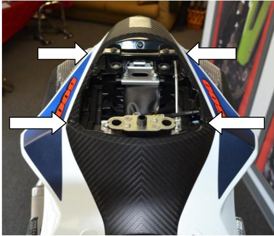
5. Remove the 4 pop rivets that are located on the top of the tail.
