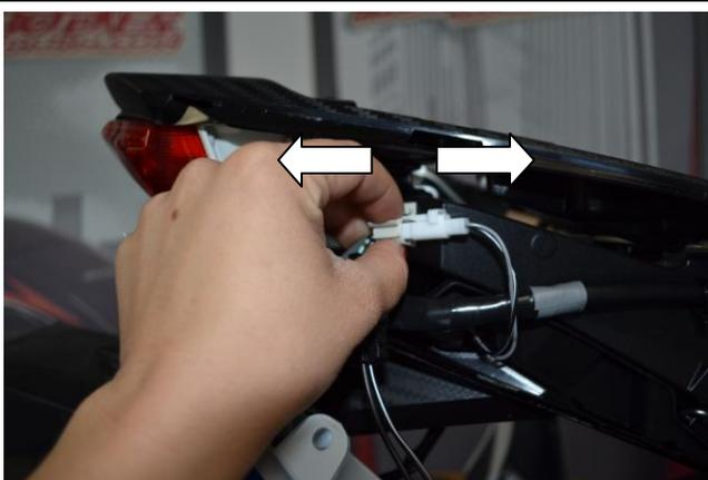
9. Disconnect the electrical running to the mud flap (located on the right side of tail).
