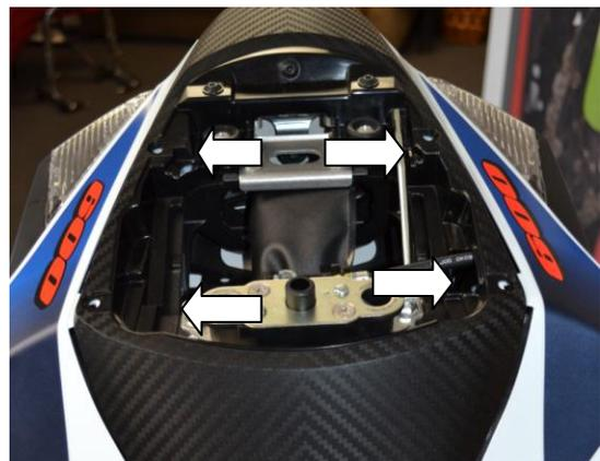
16. Reinstall 4 pop rivets that are located on the top of the tail.
