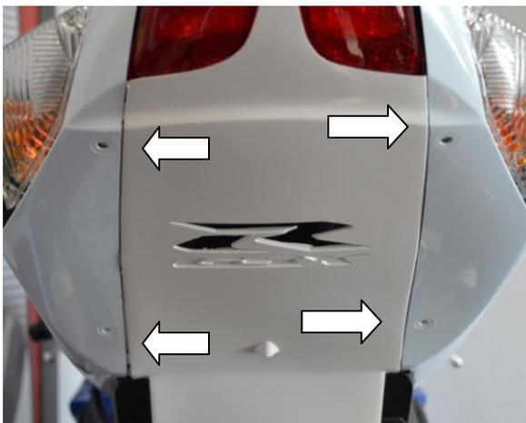
15. Reinstall 4 pop rivets on the bottom of the side tail fairings.
